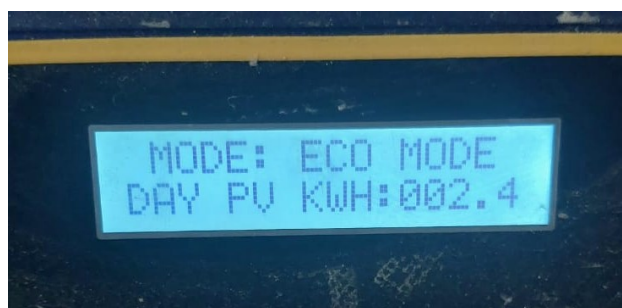
Figure 1The solar panel meter reading shows that 2.4 kWh energy was generated
