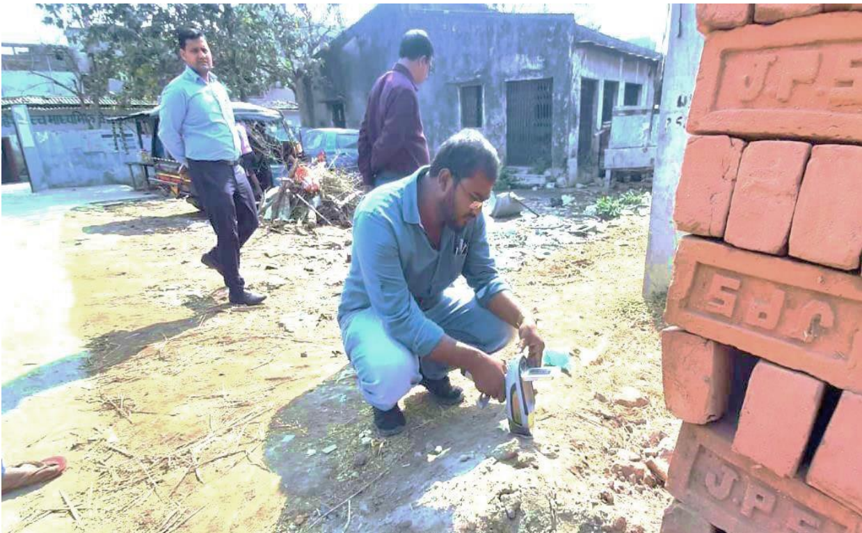
EIS officer testing soil sample for lead during survey in Patna district, Bihar, February 2020
