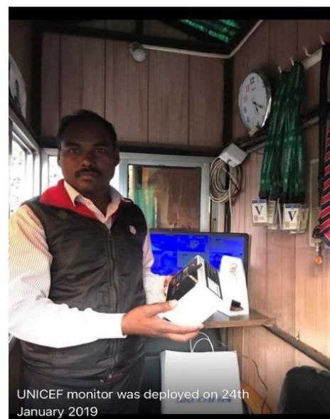
*Low cost air quality monitor has been installed for real time air quality monitoring*
